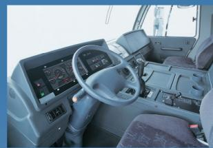
**Two-passengers, full-width cabin** The full-sized cabin accommodates two passengers. The telescoping and tilting steering wheel can be manipulated to adjust the driving position to suit the operator. Furthermore, the three-way adjustable air-suspended seat, with headrest, allows comfortable traveling for the operator.
